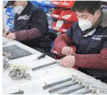
Heater Assembly Inspection and Finished Product Inspection
