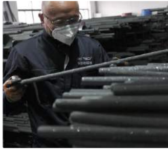
Finished product surface defects second inspection
